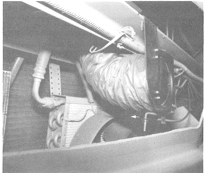
Figure 72 – Air Inlet Hose Removal: Remove the 4½"-diameter air inlet hose that is fastened to the back side of the firewall. With the inlet hose disconnected, you can begin removal of the upper air deflector. Starting with the 1981 models, the hose can be disconnected at the grille.
