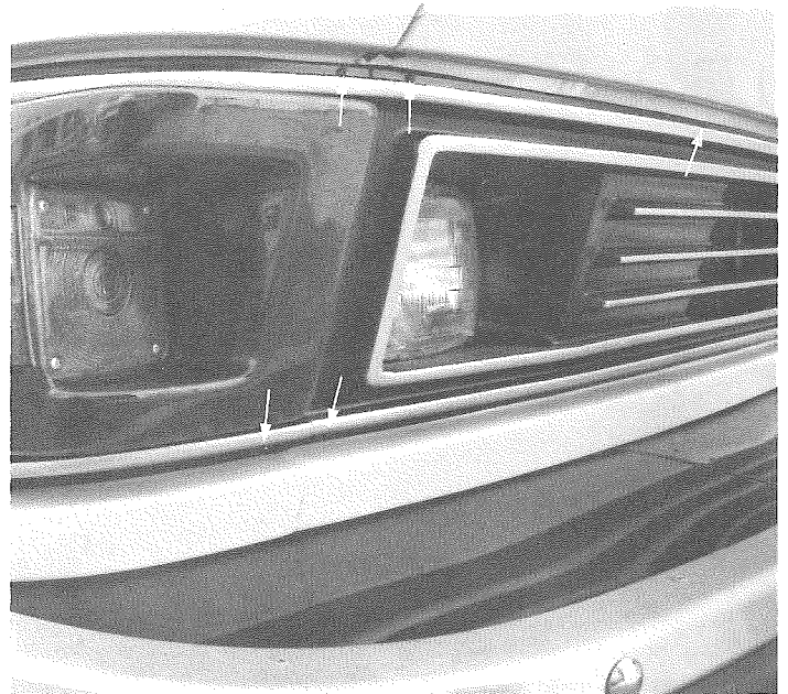
Figure 69 — Grille Removal: Remove 13 No. 6 pan head Phillips, black-painted heads. Screw locations include 3 at each end, 3 at the center, and 4 across the top.
