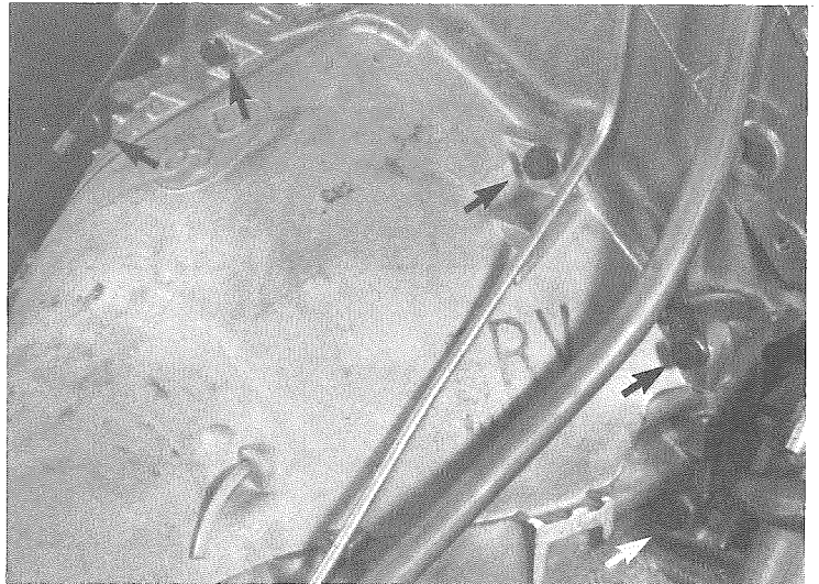
Figure 98 – BELLHOUSING – Remove the six (6) 9/16" head bolts about the bellhousing that secure the transmission to the engine.
